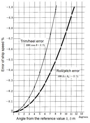
Figure4 Errors by vertical slopes in dual beams
