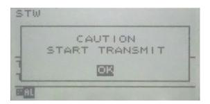
When **CLR** or **ENT** is pressed, the normal screen is displayed. Transmission starts.
