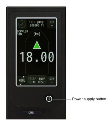
1 When the main power supply on the power board is turned on, the display unit power supply is turned on automatically.
